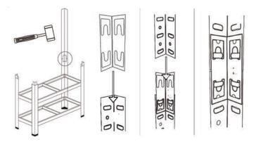
**5.** Repeat steps 2-3 to add the remaining levels. Insert MDF boards at an angle, full corners first.
