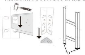
**2.** Assemble end frames with short side beams and add long front and back beams to join the frames together.
