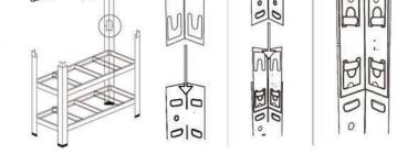
**5.** Repeat steps 2-3 to add the remaining levels. Insert MDF boards at an angle, full corners first.
