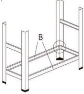
**3.** Slot the centre support beam into front and back beams.
