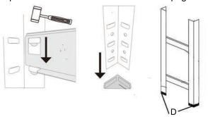
**2.** Assemble end frames with short side beams and add long front and back beams to join the frames together.
