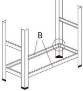
**4.** Repeat steps 2-3 to add the remaining levels. Insert MDF boards at an angle, full corners first.
