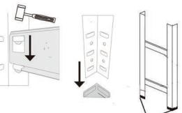
1. Slot first beam into upright. Tap into place with a 2. Assemble end frames with short side beams and add long front and back beams to join the frames together.
