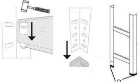
**3.** Slot upright connector into top of lower upright. Push top into place or tap down with mallet if necessary.
