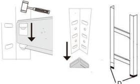
**3.** Slot upright connector into top of lower upright. Push top into place or tap down with mallet if necessary.
