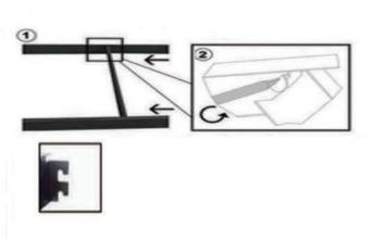
4. Insert chipboard decks onto steel frame
