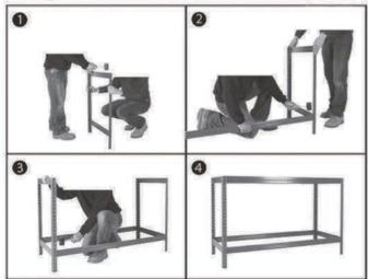
3. Slot into long beams.
