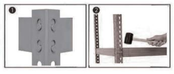
Assemble end frames with short beams & join with long front & back beams
